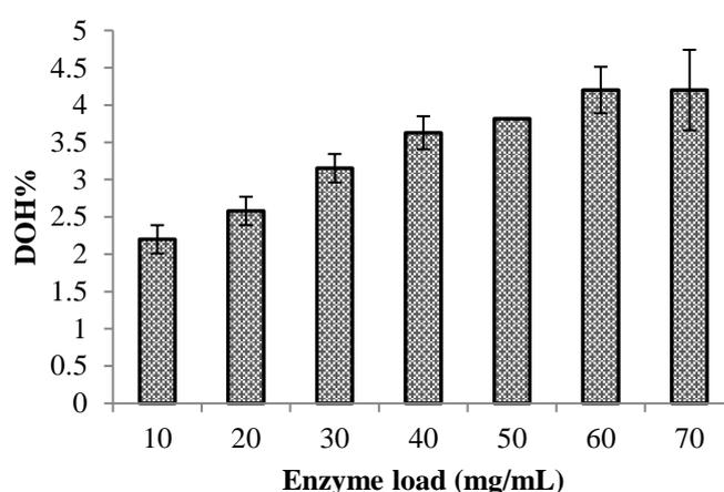
**Figure 3:** Effect of enzyme load on degree of hydrolysis [Reaction conditions: Temperature 50°C, pH 7.0, oil to buffer ratio (1:1 w/w), reaction time 15 min].
