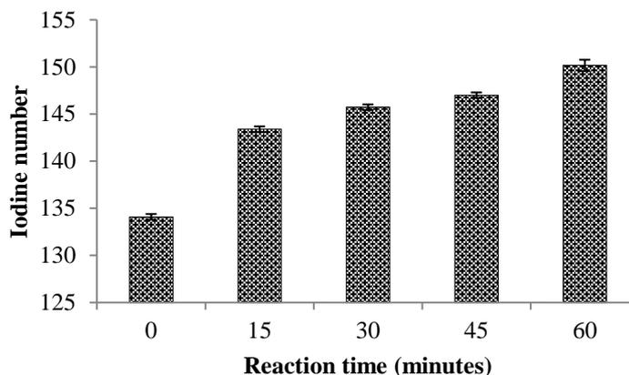
**Figure 6:** Amount of unsaturation in oil at different reaction times.
