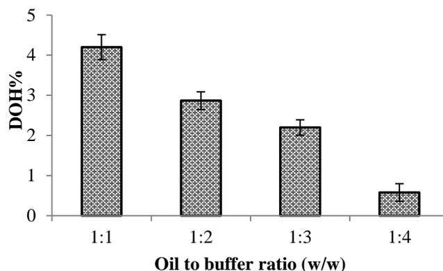
**Figure 4:** Effect of oil to buffer ratio on degree of hydrolysis [Reaction conditions: Temperature 50 °C, pH 7.0, enzyme load 60 mg/mL, reaction time 15 min].
