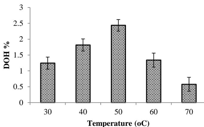
**Figure 1:** Effect of temperature on activity of CAL A [Reaction conditions: pH 7.0, enzyme load 10 mg/mL, oil to buffer ratio (1:1 w/w), reaction time 15 min].
