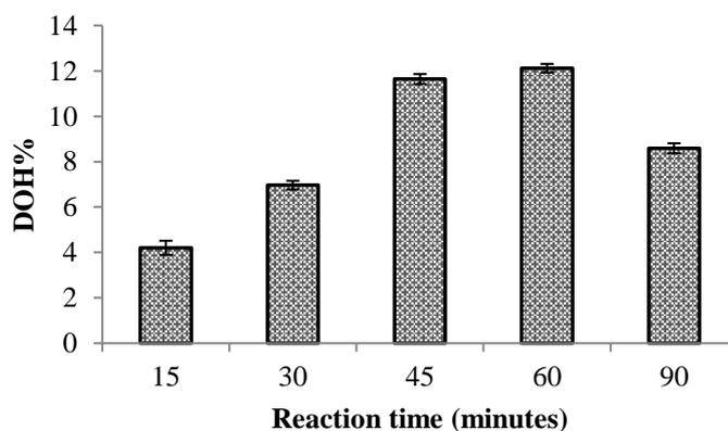
**Figure 5:** Effect of reaction time on degree of hydrolysis [Reaction conditions: Temperature 50 °C, pH 7.0, enzyme load 60 mg/mL, oil to buffer ratio (1:1 w/w)].
